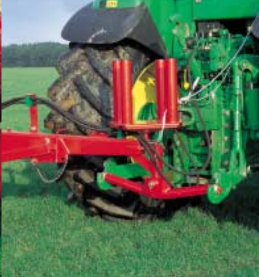
Taarup 7664 is fitted with a swivel hitch headstock. This allows wide turning angles.
