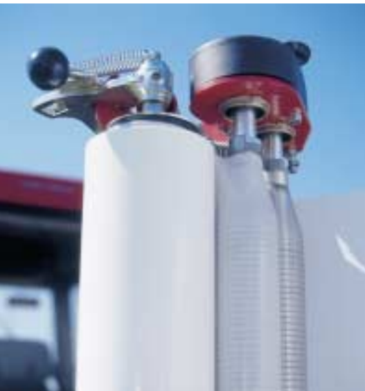
Gentle to the film Taarup bale wrappers offer a unique pre-stretch roller design with conical roller ends that keep optimum width of the stretched film. An additional benefit is that the cones are gentle to the film edges, which results in fewer problems with film tear.
