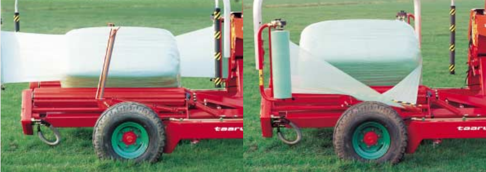
Taarup film Appli-Cutter Taarup film Appli-Cutter with sure grip keeps the stretch film ready for the next bale. This means the film is held securely while one bale is tipped off and another loaded.
