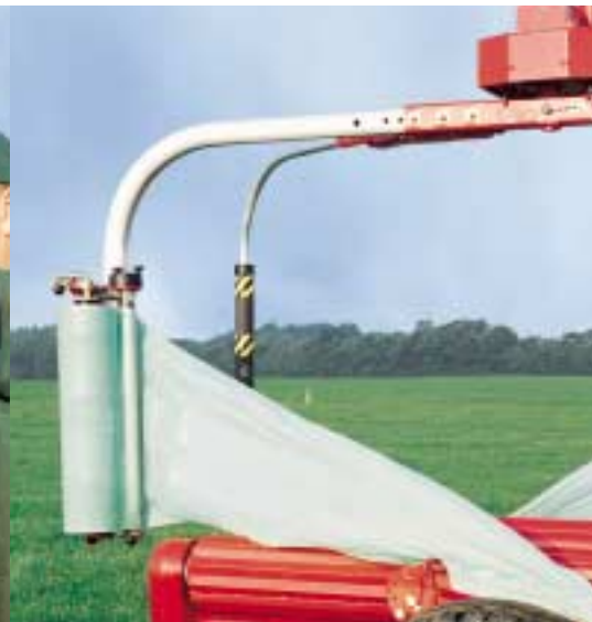
Change of film roll is quick and easy to do on a Taarup pre-stretcher. The empty core is released by pushing the upper handle sideways and upwards, in one movement. Put on the new film roll, flick the handle back into position, and the roll is then instantly locked.
