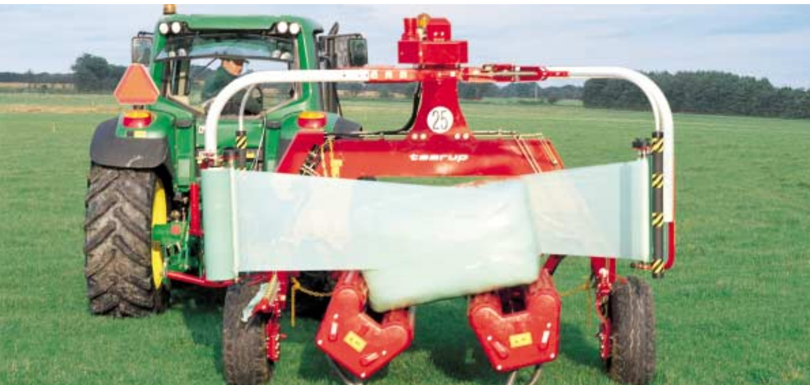
Taarup 7664 allows you to wrap on the move. Pick up one bale and wrap it as you move on to the next.
