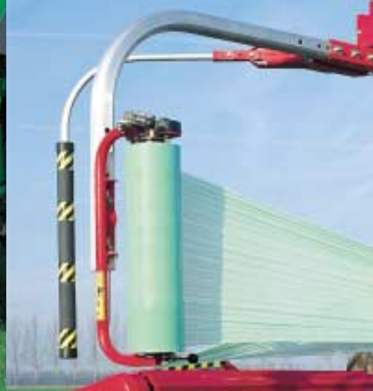
Taarup 7664 is equipped with a quick and efficient emergency stop.
