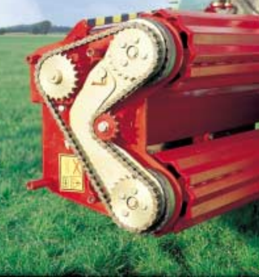
All four rollers operate via hydraulically driven heavy duty chains and sprockets.
