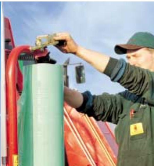
The rollers are made of aluminium, to avoid the build-up of tack from the film resulting in overstretch of film and film tear. A special pattern keeps air and water away as the film is being stretched.
